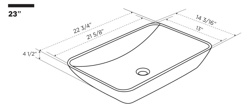
ATTENTION! Dimensions may vary by up to 3/8". It is highly recommended to pull all dimensions of actual model for installation and measuring purposes.
